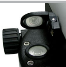
Fold-up mirror for easy alignment
