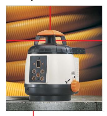
Automatic 635 nm rotation laser for indoor and outdoor applications. Rapid horizontal self-levelling. vertical alignment with adjustable foot. Pendulum system with magnetic damping and 3.5° self-levelling-range.
